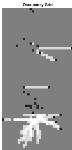
Fig. 2. Example occupancy grid map generated by two agents. The robots were placed in a 230\text{cm} \times 190\text{cm} arena. Barring walls, there were no obstacles in the environment. Each grid cell represents 10 centimeters. We used an odds value of 0.85. As in standard occupancy grid mapping, darker colors mean the cell is more likely to be occupied. We did not include our third robot in this test due to technical failure. The demo that created this map is available in our GitHub repository [1].
